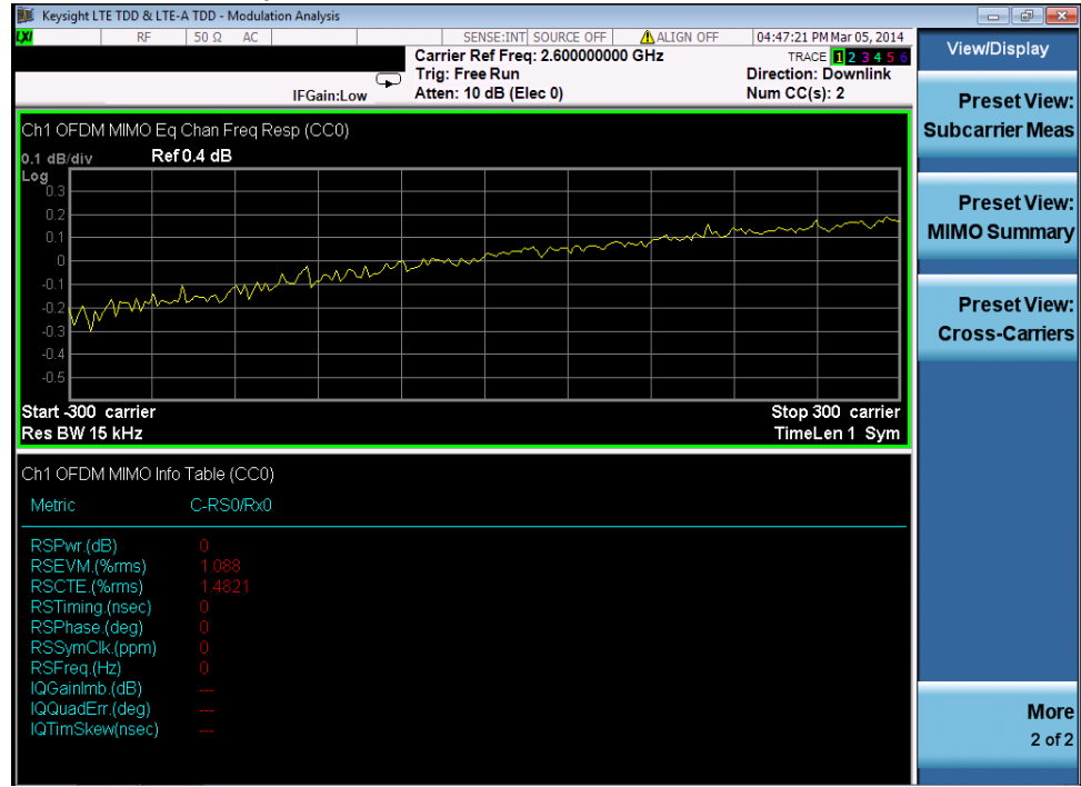
Figure 2-31 LTE TDD & LTE-A TDD Downlink Modulation Accuracy Measurement Result (Preset View: MIMO Summary)
