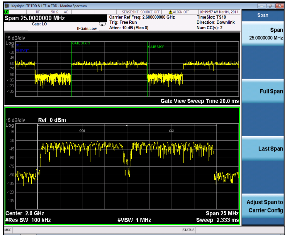
Figure 2-4 LTE TDD & LTE-A TDD Downlink Monitor Spectrum Measurement Result - Gate View On
