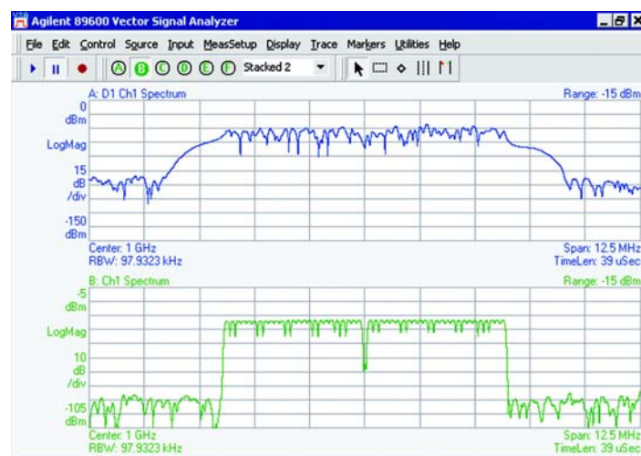
Frequency domain response of a OFDM signal without using an instrument trigger (upper trace) and using a trigger to set the beginning of the downlink frame (lower trace). (Example from the Keysight 89600).
